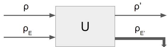
Fig. 2. In quantum computing, loss of information due to environment-induced decoherence is represented by a unitary operator U
